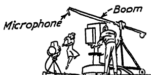
Boom for supporting a microphone out of range of a television camera.
